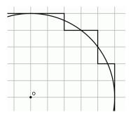
Each cell is 0.1 m x 0.1 m x 0.1 m. There are five layers of 0.1 m each, for a total height of the cylinder of 0.5 m. On each layer, the disk is replaced by 80 cells according to the picture above (showing only a quarter of the disk). If the unit is 0.1 m, the cells which are kept are those which satisfy:
